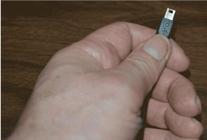
To connect the MR7 to the computer, take the supplied USB cable and orient the smaller end so that the side with the black rectangle is on top.
