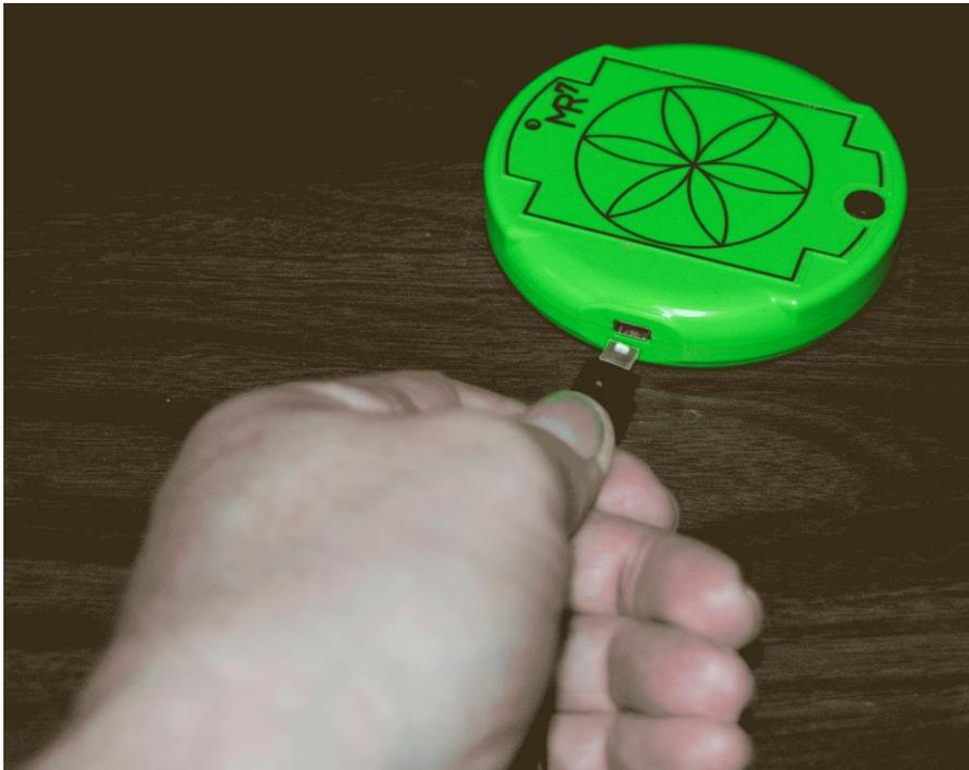
Make sure the MR7 is OFF and plug the USB cable into the MR7. The MR7 is OFF if the green LED (by the MR7 label) is not lit.
