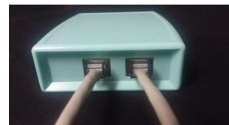
If using the two red LED light disks, plug them into the RJ45 plug jacks on the bottom of the JOINT PEMF. When using the LED lights, the lights MUST face the skin. The lights will not penetrate through cloth. The LED lights will feel warm. The lights need to breathe. Do not sandwich them between you and furniture. If the LED lights get too warm for your skin, move to another position. LEDs can be held against the skin with a brace, sock or ace bandage.
