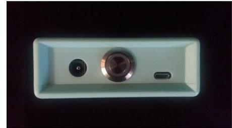
To turn the Joint PEMF device ON, Push the large On/Off button in the middle, until the lighted ring turns green. This ring will stay green while the programs are running. The Green On/Off light will turn Flashing Red when the device needs a charge. To turn the Joint PEMF device OFF, press and hold the On/Off button for about two seconds. The device will beep and turn off. If running programs when the charger is plugged in, the green light will flash.
