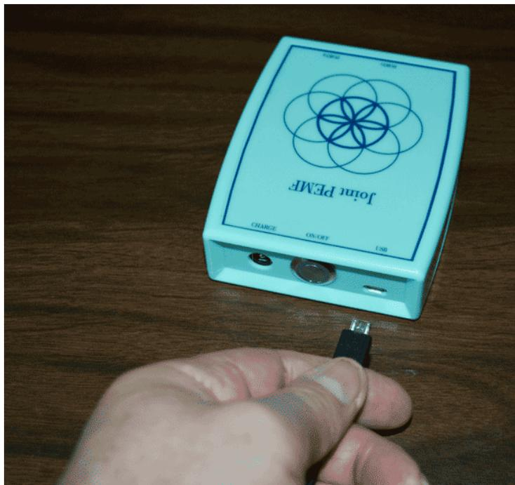
Make sure the JOINT PEMF is OFF and plug the Mini-USB cable into the mini-USB jack in the unit. The JOINT PEMF is OFF if the green LED ring light is not lit.
