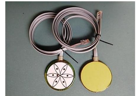
The Magnetic disks or the LED disks plug into the RJ45 jacks on the back side of the JOINT PEMF. Do not wrap the disc cables or Power cable around the JOINTPEMF device. Instead, unplug them and wrap each cable individually.
