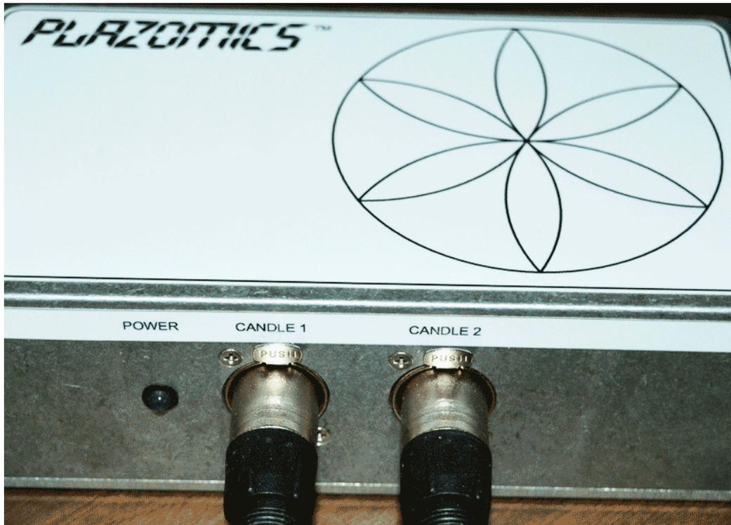
Plug the male ends of the two audio cables into the side of the PLAZOMICS unit. Make sure to push each cable in all the way until you hear a click. If you do not hear a click, the cable is not plugged in all the way.
