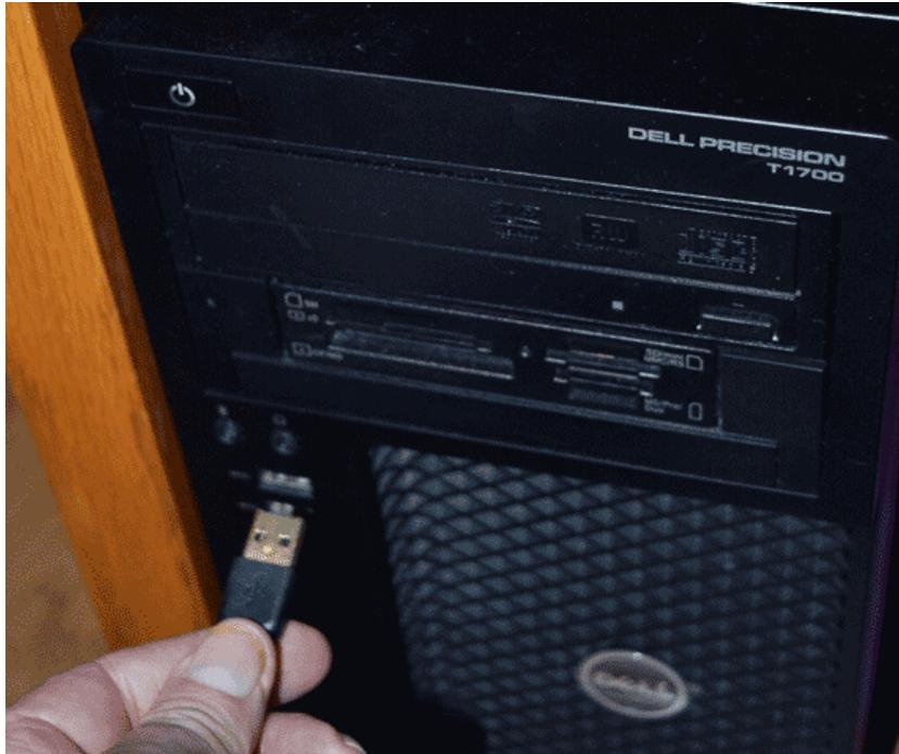
Plug the larger end of the supplied USB cable into a spare USB port on your computer.
