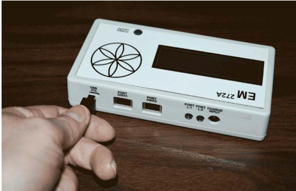
For the EM272A, make sure the unit is OFF and plug the Mini-USB cable into the mini-USB jack. The EM272A is OFF if the green LED ring light is not lit.
