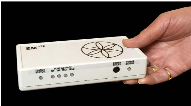
On the EM272, there are 5 lights on the left. The first one is the Charge status, (Green when fully charged; amber/red when low charge). The second and third lights show that the Nasal Probes (L and R) are attached. They glow green when in use. Lights four and five show that the Magnetic Discs (L & R) are attached. They also glow green when in use.
